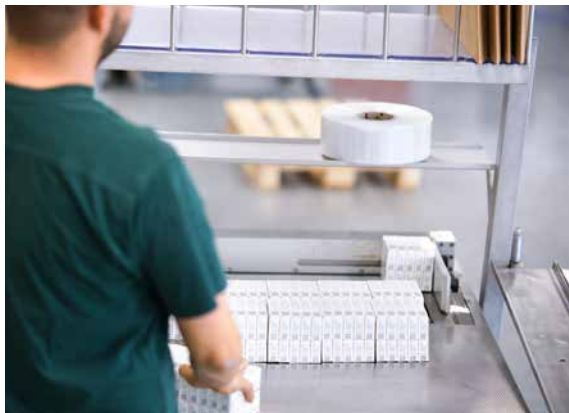
Serialized and bundled drug packages undergo final inspection and leave the packaging line.
